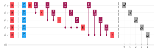
Fig. 7. Deciding whether the first vertex lies in the maximum-sized clique on the backend Manila.
