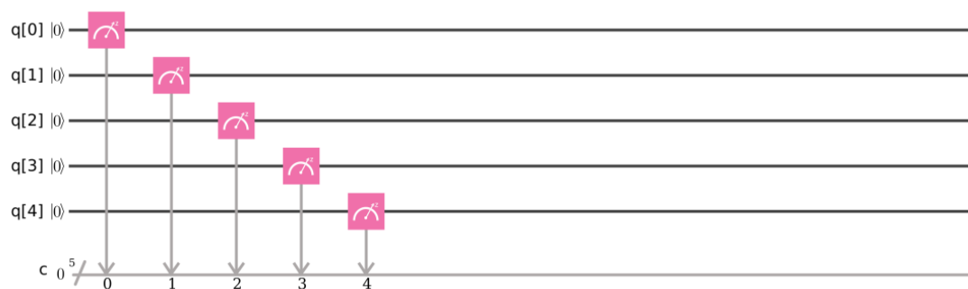
Figure 1.1: The quantum circuit of declaring and measuring five quantum bits.
