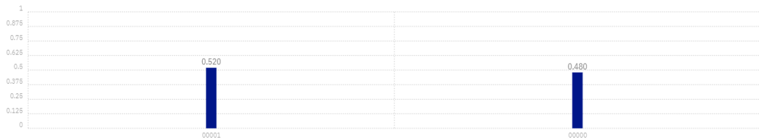
Figure 1.10: After the measurement to the program in Listing 1.5 is completed, we obtain the answer 00001 with the probability 0.520 or the answer 00000 with the probability 0.480.
