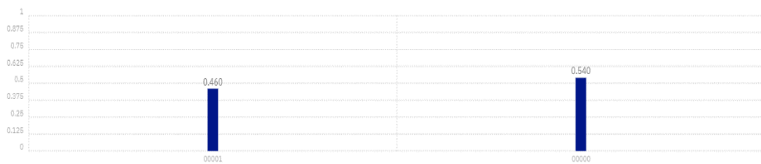
Figure 1.20: After the measurement to the program in Listing 1.10 is completed, we obtain the answer 00001 with the probability 0.460 or the answer 00000 with the probability 0.540.
