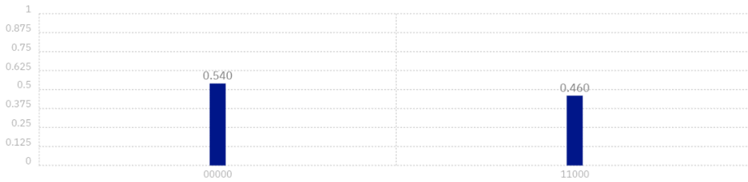
Figure 1.23: After the measurement to the program in Listing 1.11 is completed, we obtain the answer 00000 with the probability 0.540 or the answer 11000 with the
