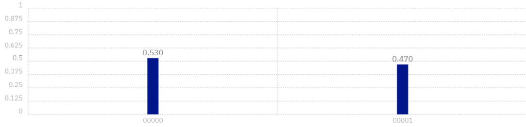
Figure 1.25: After the measurement to the program in Listing 1.12 is completed, we obtain the answer 00000 with the probability 0.530 or the answer 00001 with the probability 0.470.
