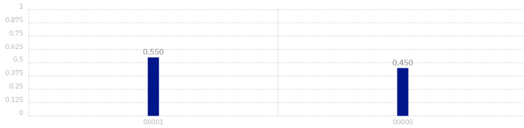
Figure 1.18: After the measurement to the program in Listing 1.9 is completed, we obtain the answer 00001 with the probability 0.550 or the answer 00000 with the probability 0.450.
