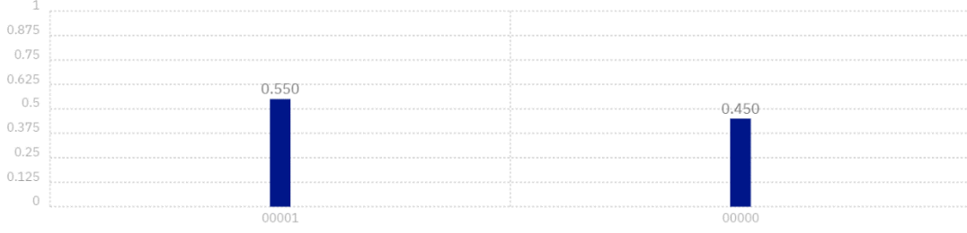
Figure 1.12: After the measurement to the program in Listing 1.6 is completed, we obtain the answer 00001 with the probability 0.550 or the answer 00000 with the probability 0.450.
