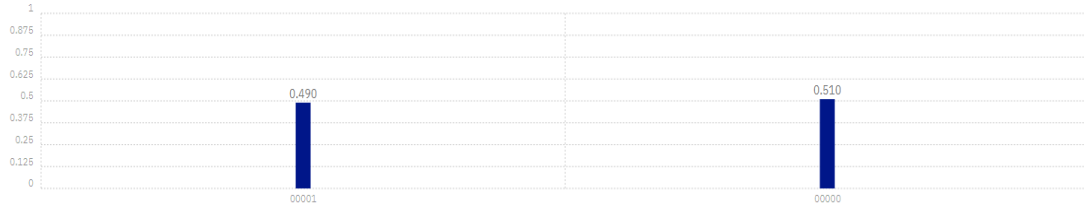
Figure 1.8: After the measurement to the program in Listing 1.4 is completed, we obtain the answer 00001 with the probability 0.490 or the answer 00000 with the probability 0.510.
