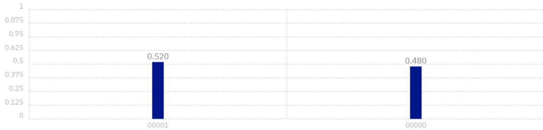
Figure 1.6: After the measurement to the program in Listing 1.3 is completed, we obtain the answer 00001 with the probability 0.520 or the answer 00000 with the probability 0.480.
