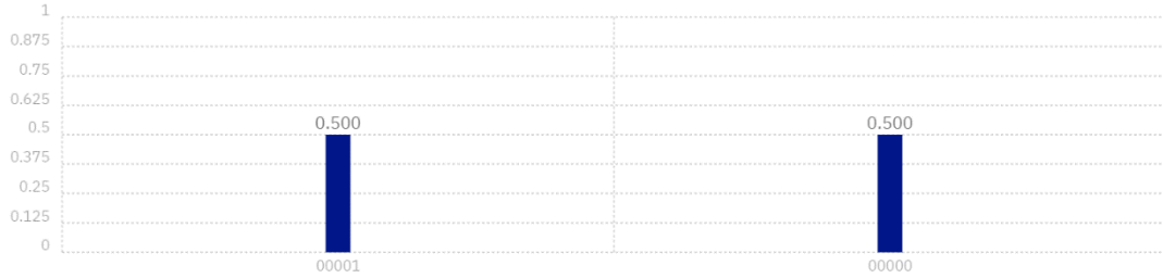
Figure 1.14: After the measurement to the program in Listing 1.7 is completed, we obtain the answer 00001 with the probability 0.500 or the answer 00000 with the probability 0.500.
